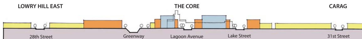
Sculpted Building Envelopes: The Plan recommends future development be sculpted to create better transitions and reduced shadowing of public spaces and streets.
