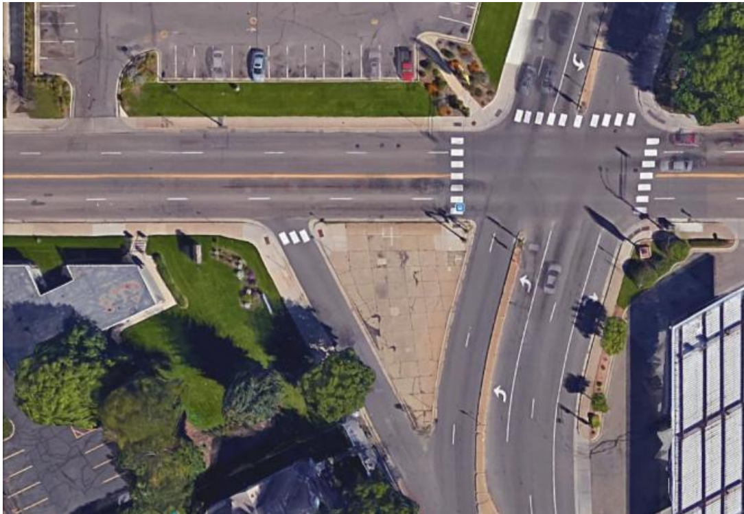
Figure 12: East Broadway Street: Elimination of Eastbound Right-Turn Channel Construction of Eastbound Exclusive Right-Turn Lane
