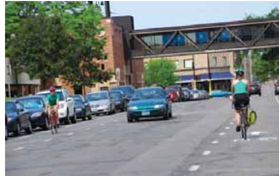
A national first: advisory bike lanes with no centerline on East 14 th Street in Minneapolis, MN
