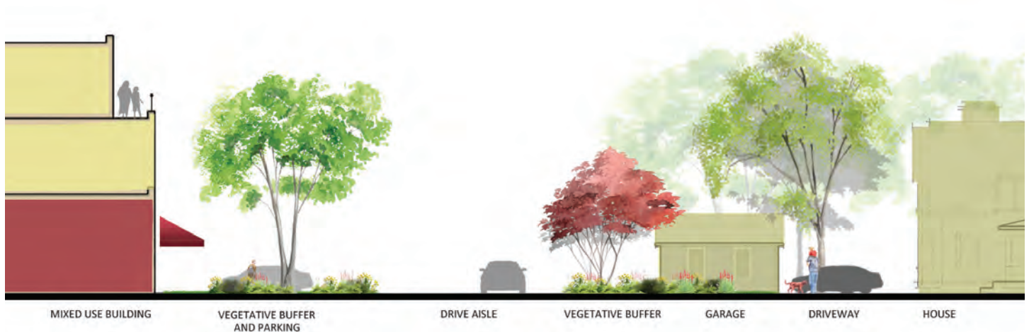
Cross section illustrating the transitional zone between the back side of 3-story development and existing single family residential featuring vegetative buffers, a drive aisle and no alley.
