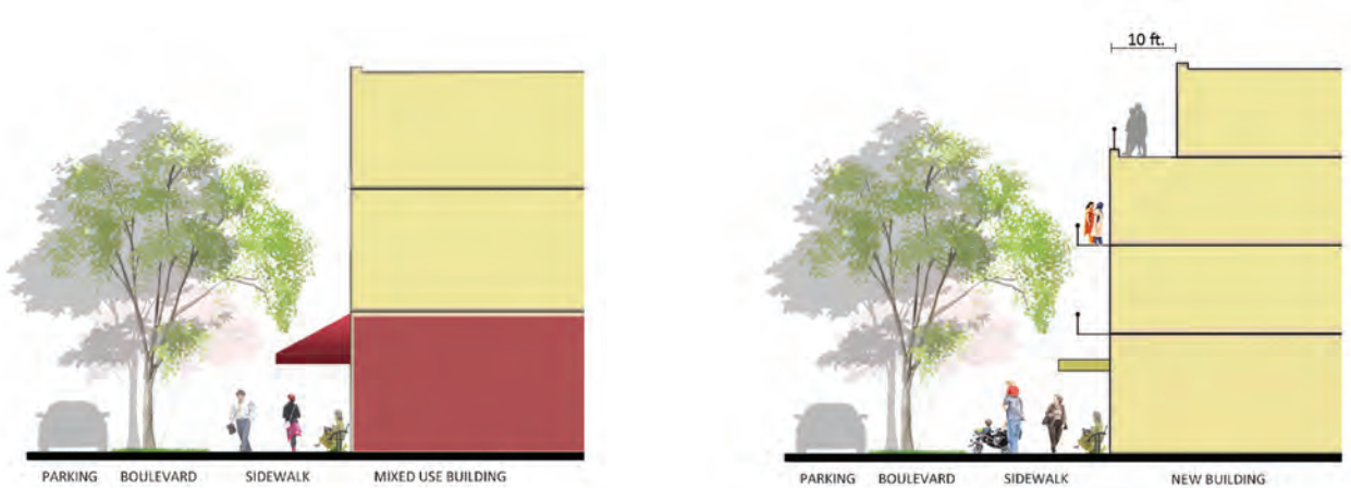
Cross section of two buildings illustrating a new 3-story, mixed use building and a new 4-story, multifamily building with the upper story stepped back from the front facade.
