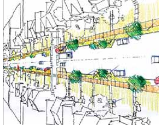
Washington St: Improved for transit • Nice bus stops • Traffic calming: narrowed lanes • Safer crossings • Stormwater management along curbs
