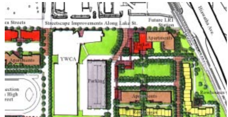
Shared parking strategies and remote parking strategies could be applied though increasing parking capacity at the YWCA and parking facilities associated with future redevelopment of the Hi-Lake Shopping Center. Cost effective underground parking could be built under the public green to support higher density development on the Edison/PPL site and providing parking for the public market.
