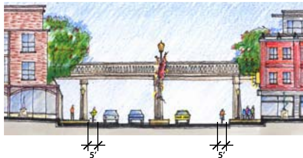
Section BB: Proposed arrangement of bike and auto lanes on Central Avenue, between 7th Street SE and 18th Avenue NE.
