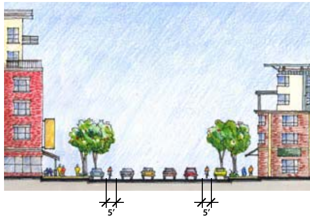
Section AA: Proposed arrangement of bike and auto lanes on Central Avenue, between 27th Avenue NE and 18th Avenue NE.
